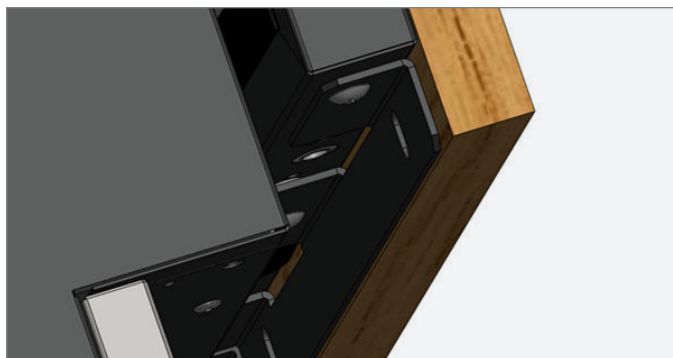
FIG. 4. The bottom edge of the panel should align with the bracket as shown.
