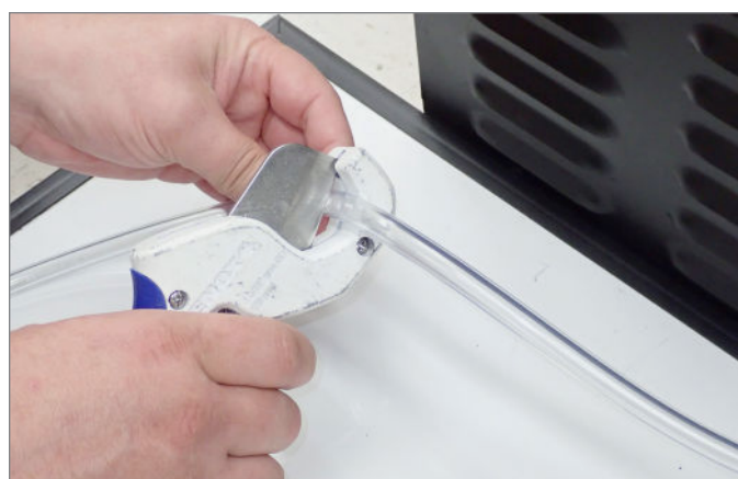
FIG. 3. Cut the drain line with tubing cutters.
