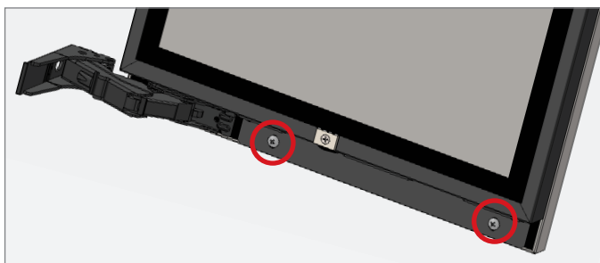
FIG. 2. Bottom door bracket screw locations.
