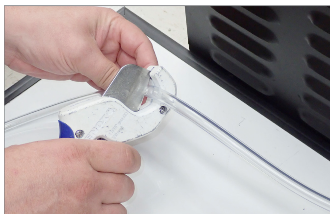
FIG. 3. Cut the drain line with tubing cutters.
