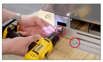
FIG. 8. Anti-tip bracket shipping bolt locations. Other side not shown.
