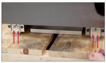
FIG. 7. Shipping bracket bolt locations.
