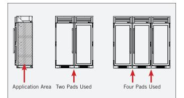
FIG. 14. Install foam pads between the joined units.
