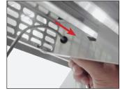
**FIG. 6.** Remove the p-clip holding the wire to the rainshield.
