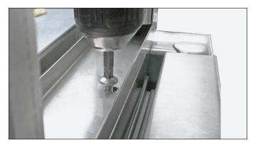
FIG. 10. Remove the screws from the metal channel.
