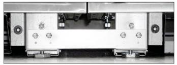
FIG. 18. Installed joining bracket.
