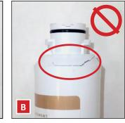
**FIG. 4.** Undamaged water filter head (A) vs. a damaged water filter head (B).
