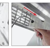
**FIG. 6.** Remove the p-clip holding the wire to the rainshield.
