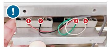
FIG. 20. Connect the reed switches with the original wire configurations.
