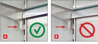
FIG. 5. Underside view. Left side shown.A: CORRECT; Bottom tab is fully seated in the shelf standard.B: INCORRECT; Bottom tab is not seated in the shelf standard.
