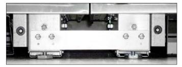
FIG. 18. Installed joining bracket.
