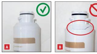
FIG. 5. Undamaged water filter head (A) vs. a damaged water filter head (B).
