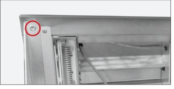
FIG. 8. Bracket screw location. Other bracket not shown.
