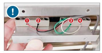
FIG. 5. Label the original wire locations **BEFORE** disconnecting the reed switch.
