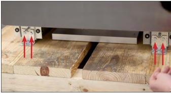
FIG. 7. Shipping bracket bolt locations.
