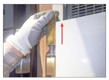
FIG. 2. Remove the hinge covers.
