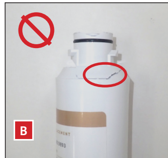
FIG. 5. Undamaged water filter head (A) vs. a damaged water filter head (B).
