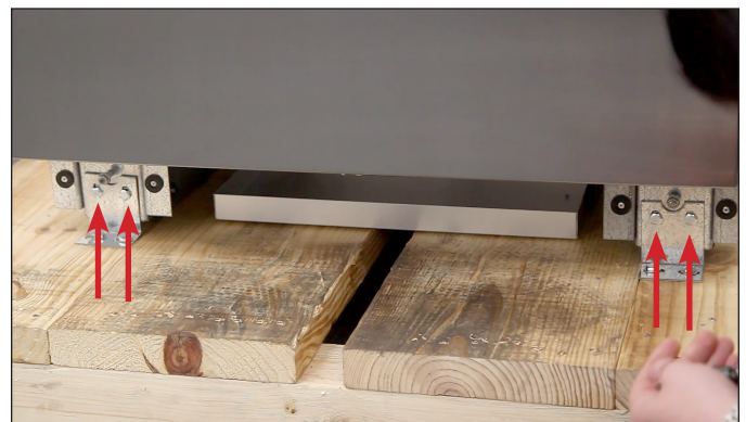
FIG. 7. Shipping bracket bolt locations.
