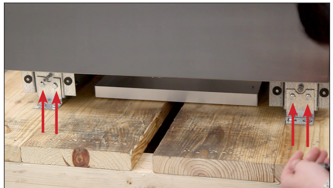
FIG. 7. Shipping bracket bolt locations.
