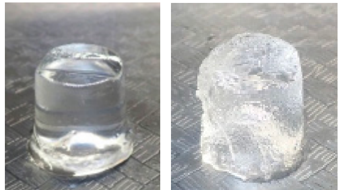
FIG. 2. Ice deteriorates and roughens as it ages.
