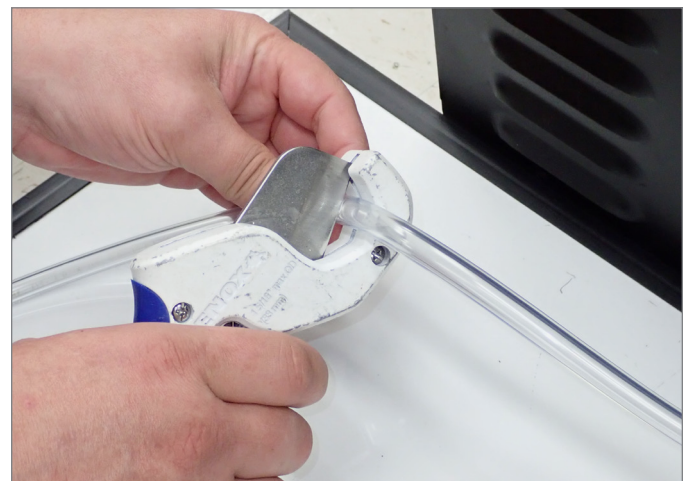
FIG. 3. Cut the drain line with tubing cutters.
