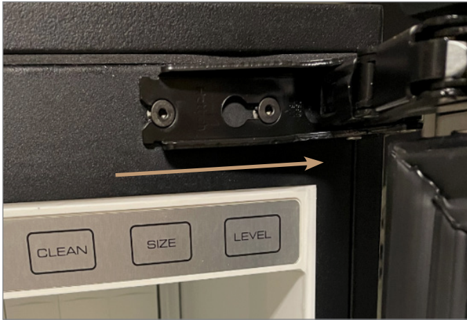
FIG. 1. Slide the door off the hinge bolts through the keyhole slots.
