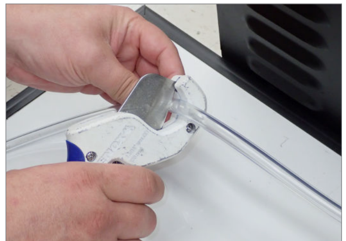
FIG. 3. Cut the drain line with tubing cutters.
