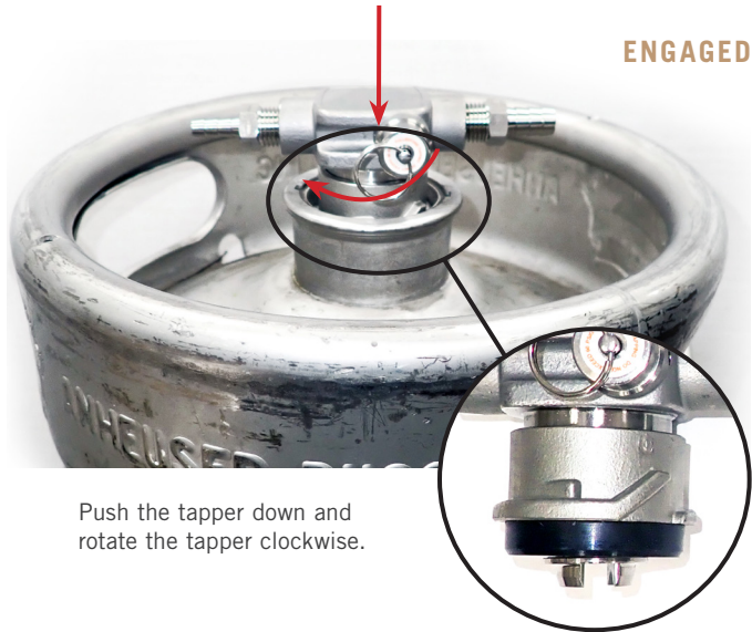
FIG. 10. Installed and connected tap. Be sure the hose clamps are tightened to prevent leaks.
