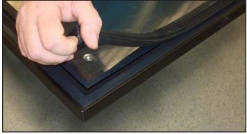
Image 2. Remove gasket from front drawer panel.
