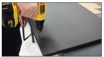
Image 6. Pre-drill holes through door front.
