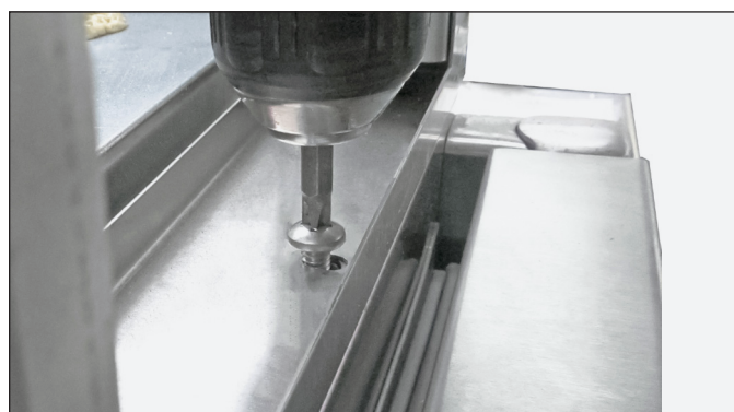
FIG. 10. Remove the screws from the metal channel.
