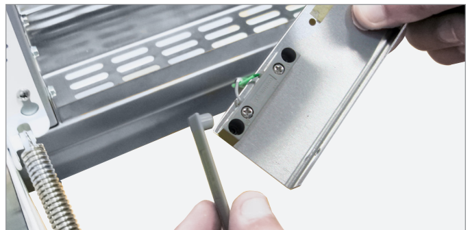
FIG. 4. Remove the plastic cover.
