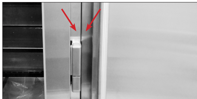
FIG. 15. Verify the cabinet fronts are flush. Adjust the units accordingly.
