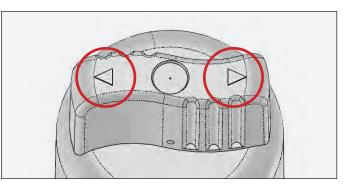
FIG. 5. Water filter handle arrow locations.
