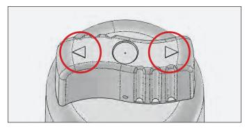
FIG. 3. Water filter handle arrow locations.
