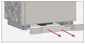
FIG. 1. Pull the kickplate from the cabinet.
