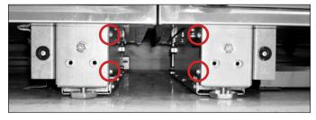
FIG. 17. Return the magnet bracket screws to their original locations
