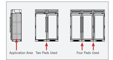
FIG. 14. Install foam pads between the joined units.
