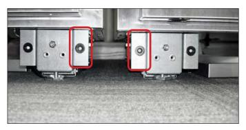
FIG. 11. Remove and discard the interior magnet brackets.
