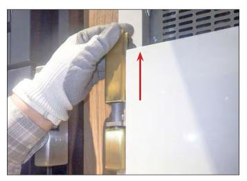
FIG. 2. Remove the hinge covers.
