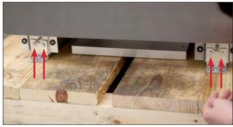
FIG. 7. Shipping bracket bolt locations.
