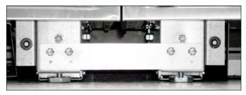
FIG. 18. Installed joining bracket.
