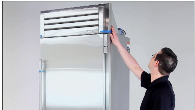
FIG. 2. Inspect the unit's exterior for visible damage.
