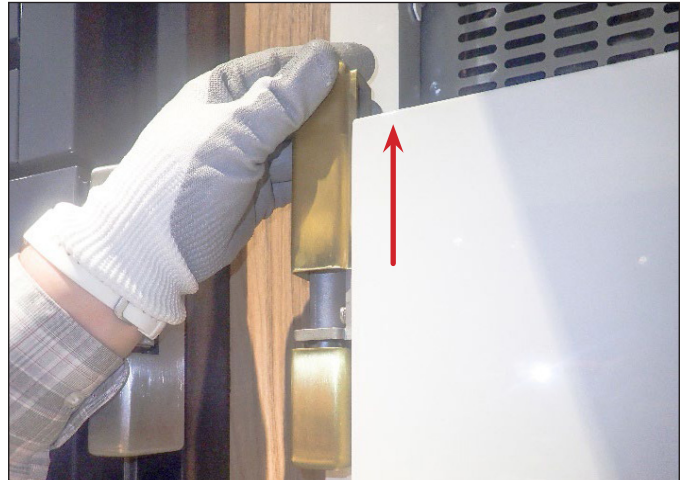
FIG. 2. Remove the hinge covers.
