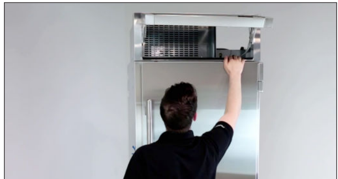
FIG. 3. Be sure to inspect the rainshield.
