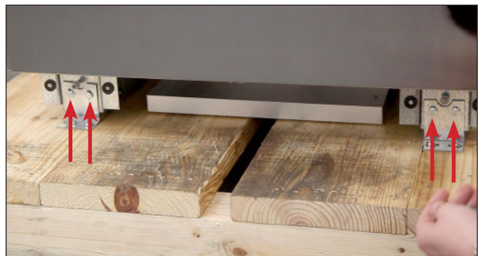
FIG. 7. Shipping bracket bolt locations.
