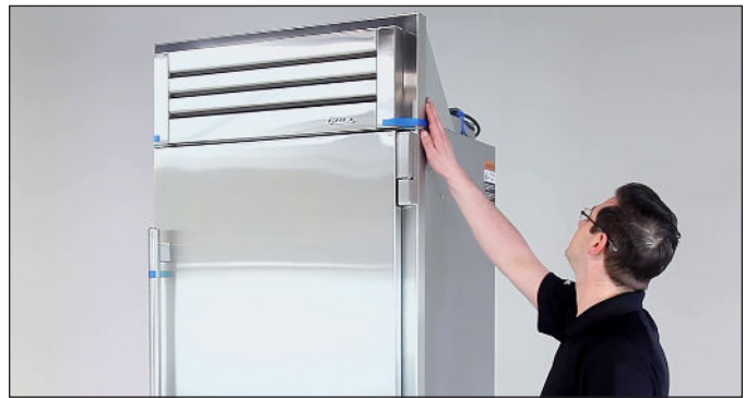
FIG. 2. Inspect the unit's exterior for visible damage.
