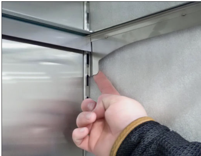
FIG. 6. Push the bottom tab inward.
