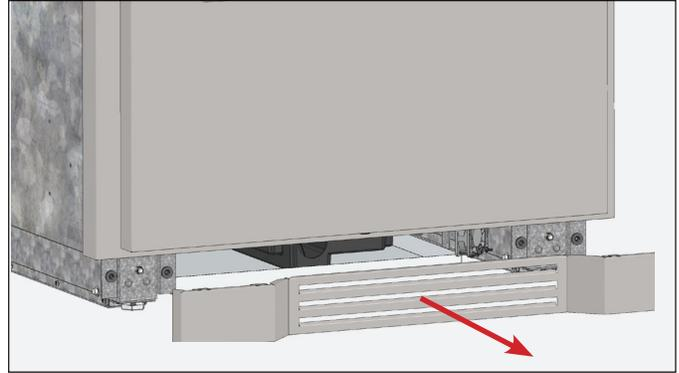
FIG. 1. Pull the kickplate from the cabinet.
