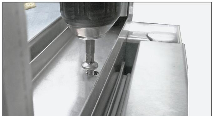
FIG. 10. Remove the screws from the metal channel.
