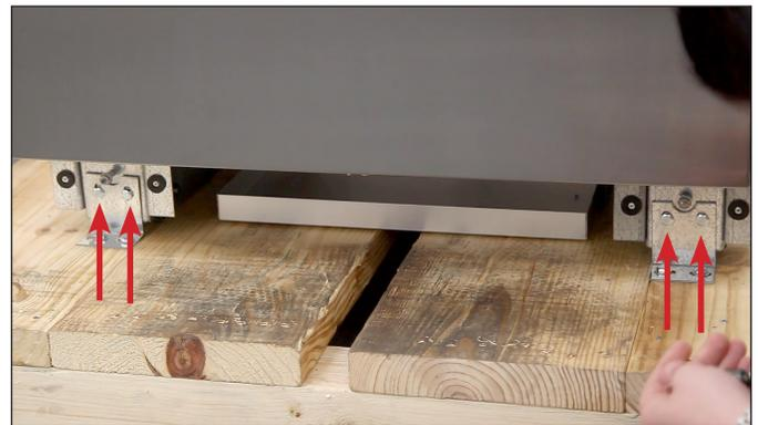
FIG. 7. Shipping bracket bolt locations.
