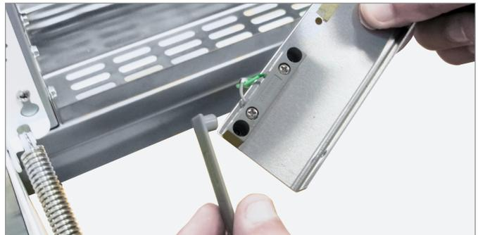
**FIG. 4.** Remove the plastic cover.
