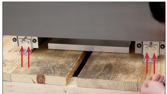
FIG. 7. Shipping bracket bolt locations.
