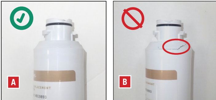
FIG. 5. Undamaged water filter head (A) vs. a damaged water filter head (B).
